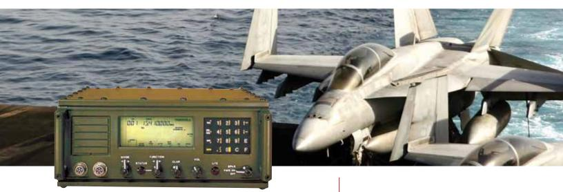
The RT7000 is a rugged, 1.6 to 30 MHz, HF/SSB transceiver designed to provide long distance voice and data communications. The RF output power is rated at 125W, PEP, and 100W, average, and there is complete protection against antenna mismatch. Modes include USB, LSB, CW, and AME; and up to 1000 preset memory channels are available.
